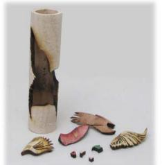
before gluing. I prefer 2-part epoxy to glue the brass tube in place. Never use polyurethane (Gorilla) glue with these inlay kits as the expansion while curing could seep through the glue joints of the inlay. Insert the brass tube so that the pheasant is centered. Once all glue has cured, sand the ends flush to the brass tube (don't use a barrel trimmer) and mount on the lathe for turning and finishing. E-mail me at kallenshaan@cox.net with any
