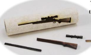
This radius will go in the upper right corner of the recess. Next fit the scope and finally the small white piece of maple under the scope. Once all pieces are in place remove the brass tube and secure the pieces with thin CA glue.
