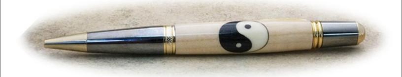
There's a total of 5 pieces in this inlay kit. To start, temporarily slide the brass tube from your pen kit (not included) into the maple background cylinder. Now insert the white and black pieces inside the circle cutout followed by the small black and white dots. Secure with the supplied elastic bands. Remove the brass tube and apply thin CA glue to all of the seams in the pattern.
